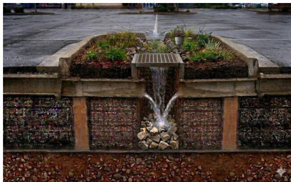
Figure 1: Geosynthetic Based Rain Garden Elevation View
