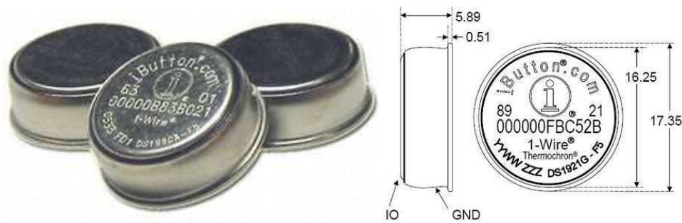
Figure 3.1: Outer Shell (left) and Dimensions (right) of Typical I-button (EDS 2012)
