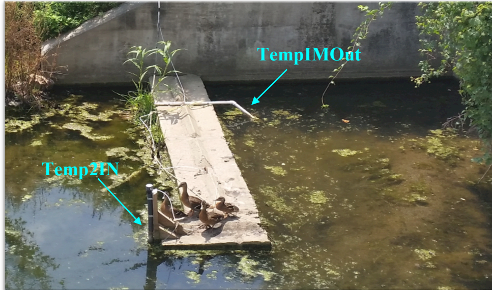
Figure 3-5: Locations of inlet temperature instruments
