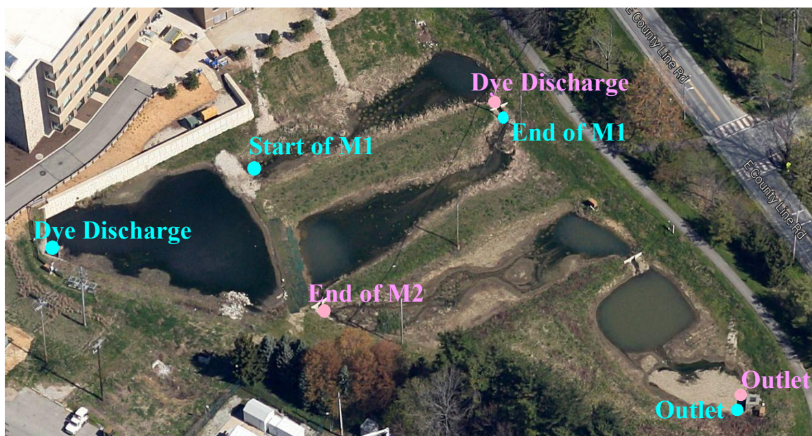
Figure 3-7: Locations of rhodamine dye discharge and Cyclops-7 sondes (Blue and pink indicate where the dye was released and its corresponding sonde locations for the matching color)
