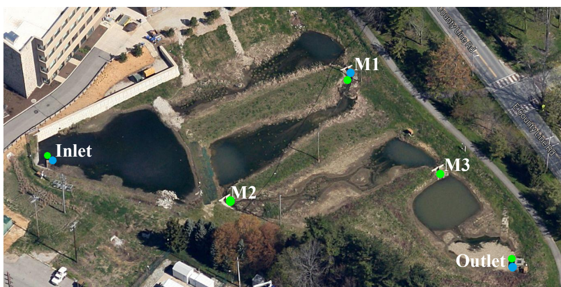
Figure 3-11: Baseflow and autosampler storm event water quality sampling locations (Green is baseflow and Blue is storm events)
