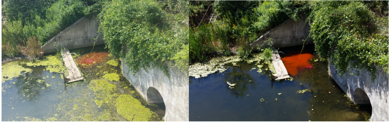
Figure 4-3: August 8 th (left) and August 28 th (right) dye release at inlet
